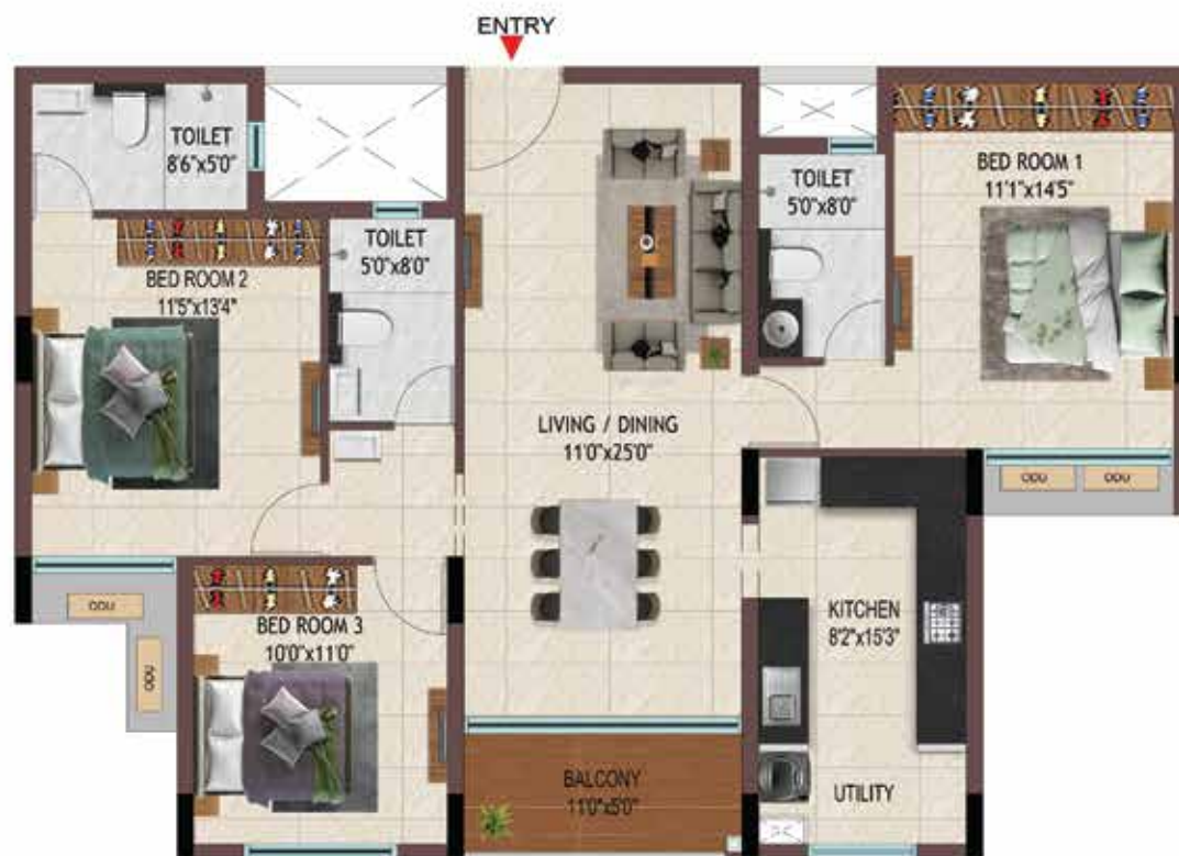
TYPICAL FLOOR (GF TO 5TH)
